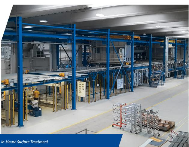
In surface treatment, we implement a modern, fully automatic machine for tartaric sulphuric acid anodising, complemented by automated spray coating machinery. Components with complex geometries or special applications, such as the BR 127, can be manually coated.
